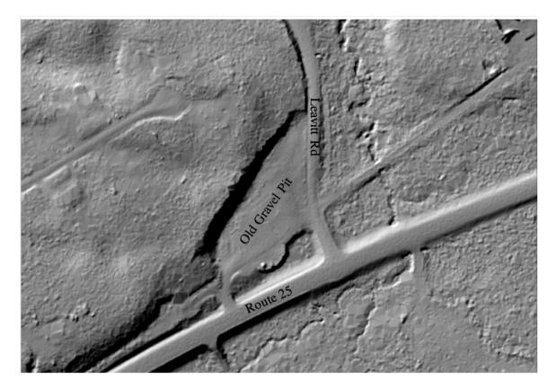
LIDAR (Light Detection and Ranging), an established remote sensing technology that measures distances with reflected laser light, graphically shows the extent to which the proposed gas station site was mined for gravel, making already-transmissive soils hypervulnerable to contamination. *Map: Dr. Robert Newton*
