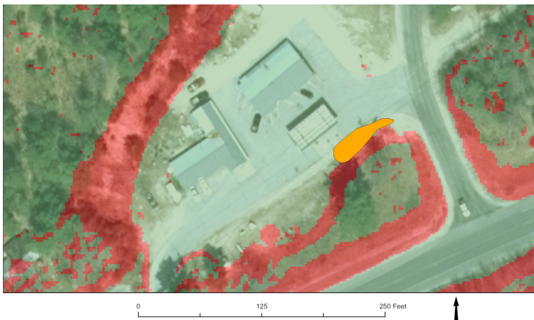
Figure 3. 2015 orthophoto of the Meena site. The bioretention basin (orange) is located directly adjacent to steep slopes (red) as determined from LiDAR data obtained from the New Hampshire Granite GIS site. The basin should be relocated at least 50 ft from these steep slopes.
