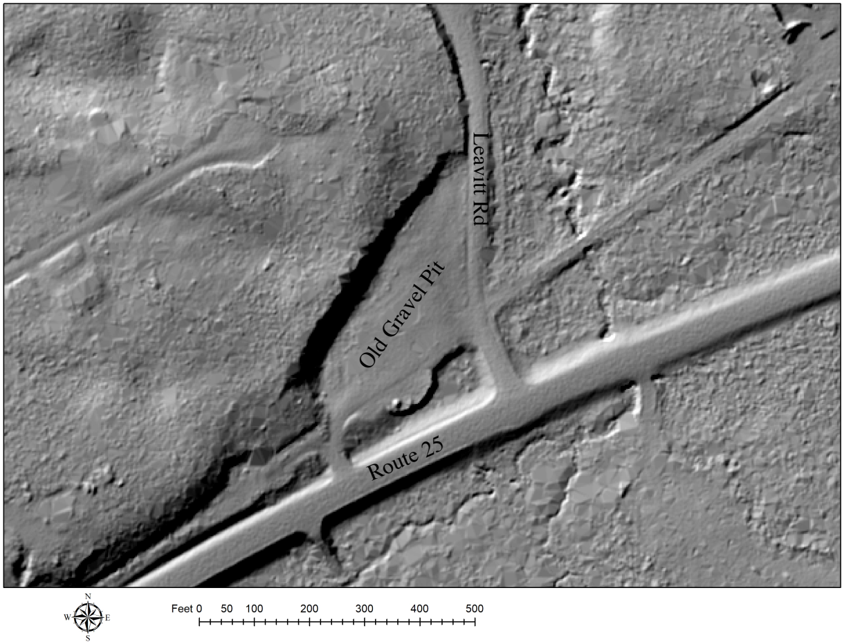
Figure 4. This is a topographic hillshade made from a LiDAR based Digital Elevation Model (DEM) with the sun located 45^{\circ} above the horizon on a 315^{\circ} azimuth. It clearly shows the extent of the gravel pit, where the proposed gas station is located. This makes this site extremely sensitive to contaminating the underlying groundwater.
