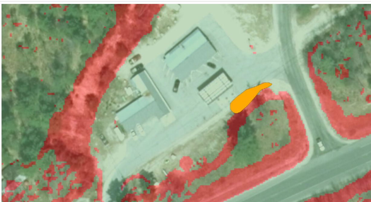
Meena’s proposed bioretention basin, in orange, is adjacent to steep slopes, in red, and is within a High Load Area, both of which would violate state regulations.
