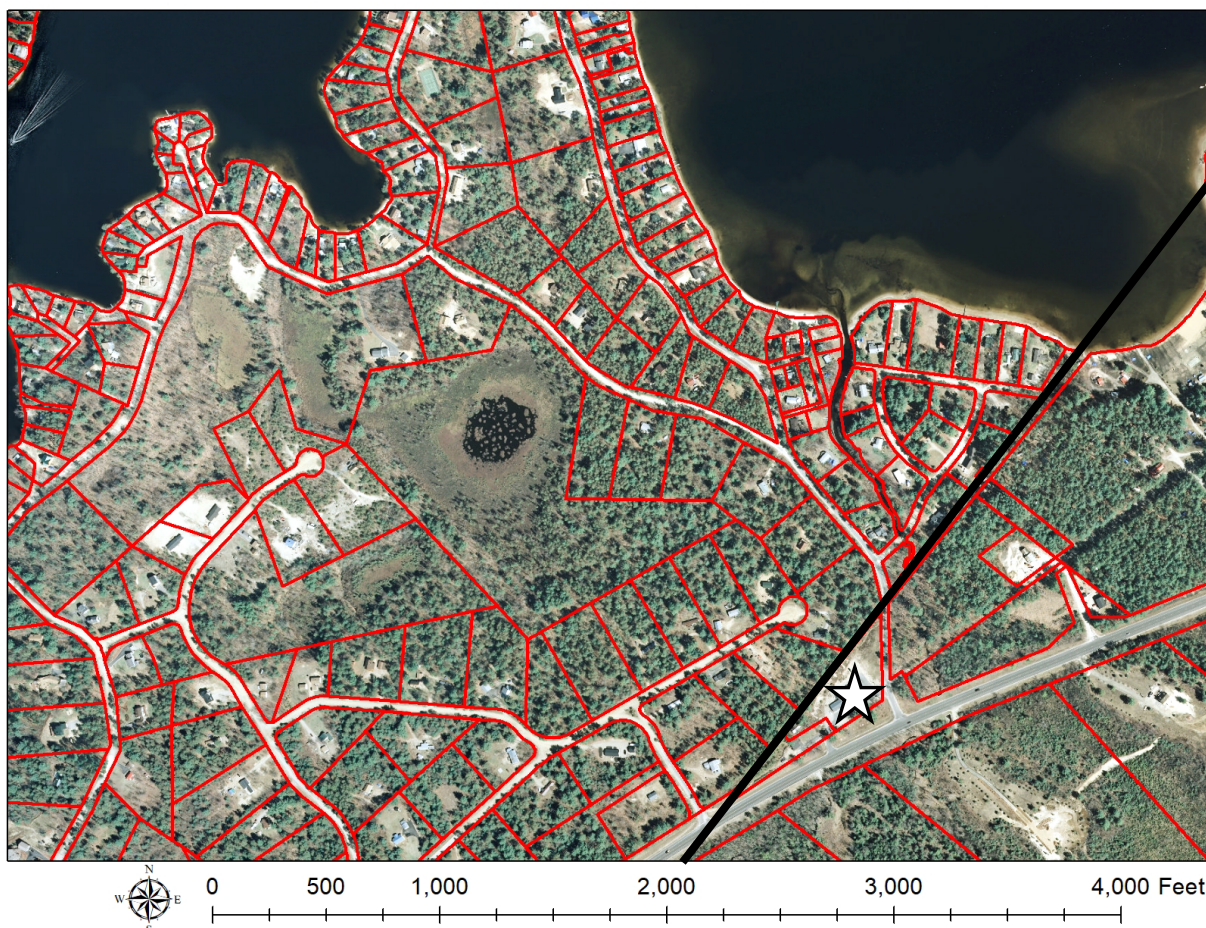
Figure 5. This is an orthophoto taken in 2006 with parcel data showing the property boundaries. The star is located at the Meena site and the black line shows the Ossiipee – Effingham town line. Groundwater flow from the Meena site is generally northward and all properties north of the site are serviced by private wells. All these properties could be impacted from a spill at the Meena site.
